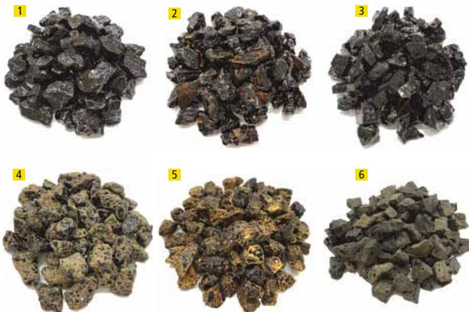
ABOVE: 1. Basalt aggregate - with anti-stripping agent 2. Lime aggregate - with anti-stripping agent 3. Slag aggregate - with anti-stripping agent 4. Basalt aggregate - no anti-stripping agent 5. Lime aggregate - no anti-stripping agent 6. Slag aggregate - no anti-stripping agent
