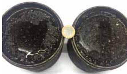
Ice formation on Marshall specimens; ice on the specimen containing Winterpave (left) was easily detached, whereas the ice on the other was not
