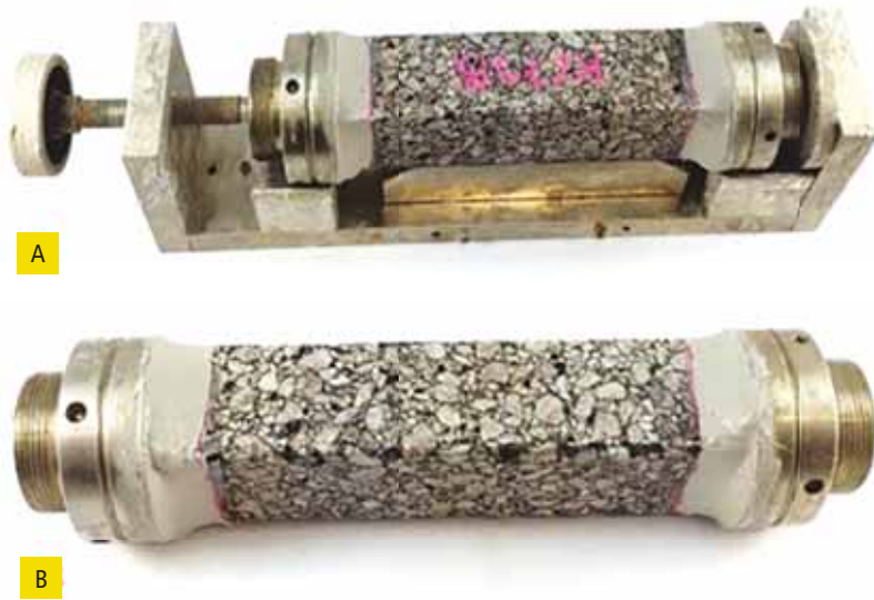
Figure 1. Typical TSRST test set-up and theory
